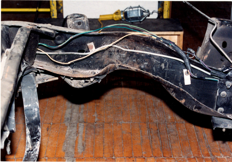
33. Close-up view of the left frame rail adjacent to the site of the CNG tank failure
